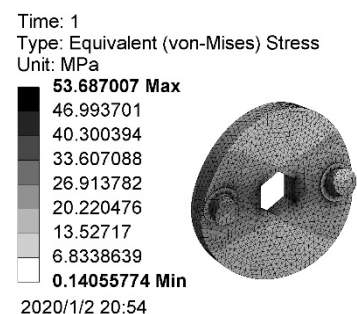
Fig. 6 Maximum stress nephogram of Drive Plate when opening time is 350ms
